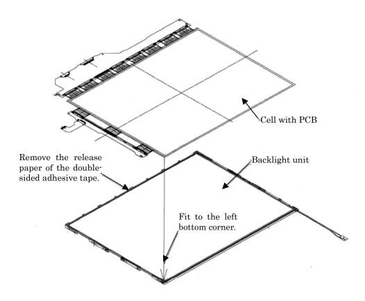
Figure 4-57 Replacing TMD fluorescent lamp (WXGA) (7)
